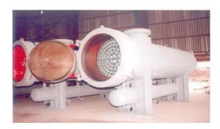
Particles that remain suspended will encounter the filter coalescer elements, which provide maximum surface area for solids retention. Liquid particles collide with and adhere to the fibers or other droplets and coalesce. Two mechanisms are involved in this action: deposition by impaction and by diffusion. The agglomerated liquid is then forced thru the media by the drag of the gas for subsequent removal by the second stage separator.
